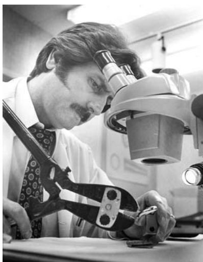
Examining Bolt Cutter Toolmarks in CCCO Lab - 1980
