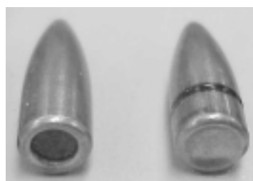
Oblique base views of the H.P. bullet from Ulyanovsk (left) and the jacketed soft point bullet from Barnaul (right)
