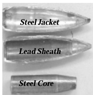
Sectioned Soviet M43 Ball Round
