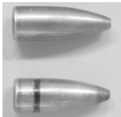
Jacketed hollow point bullet from Ulyanovsk (top) jacketed soft point bullet from Barnaul (bottom)
